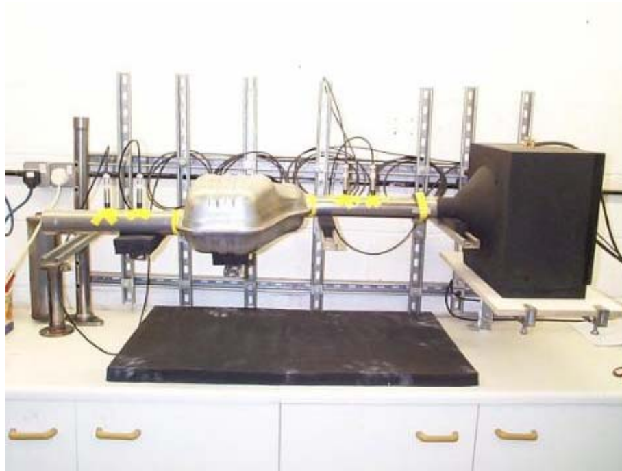
Transmission loss test equipment
